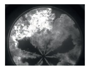
Analysis of spray vaporization with laser induced fluores-cence (LIF).
